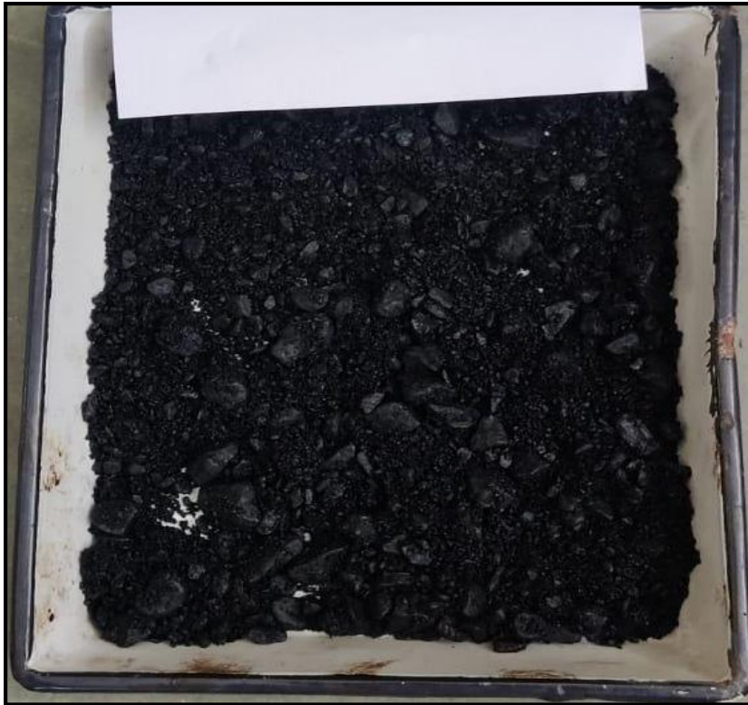
Aggregates coated with bio-bitumen
