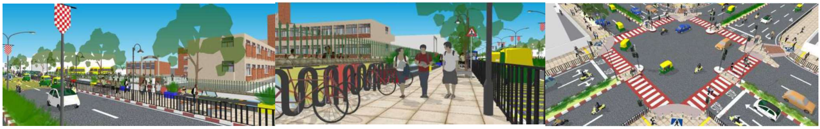
Walking Infrastructure-Footpath, Guard Rail, Pedestrian Crossing, Refuge Islands
