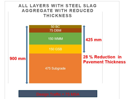
STEEL SLAG ROAD WITH REDUCED THICKNESS
