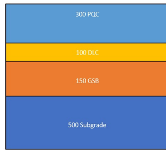
STEEL SLAG ROAD WITH REDUCED THICKNESS
