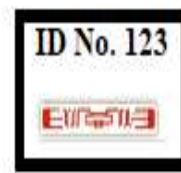
Student ID card with UHF RFID tag
