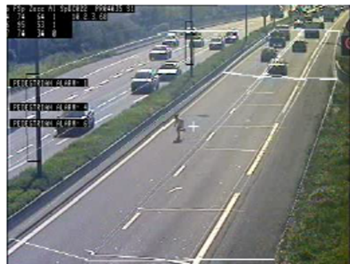
Detection of a pedestrian on a highway. Video detection can distinct vehicles, persons and objects (lost cargo, debris)
