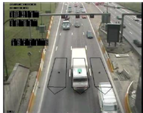
Outdoor data collection on highway: speed, occupancy, count, classification
