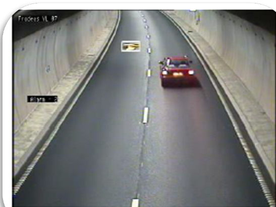
Detection of fallen object in tunnel
