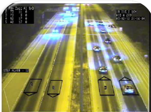
Detection of stopped vehicle on highway at night in bad weather
