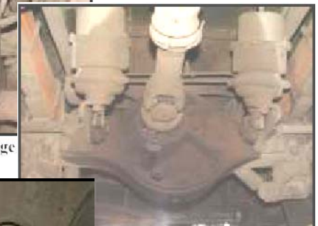
Differential Oil leakage
