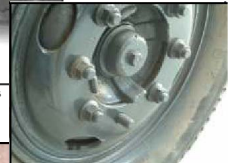
Missing Wheel nut
