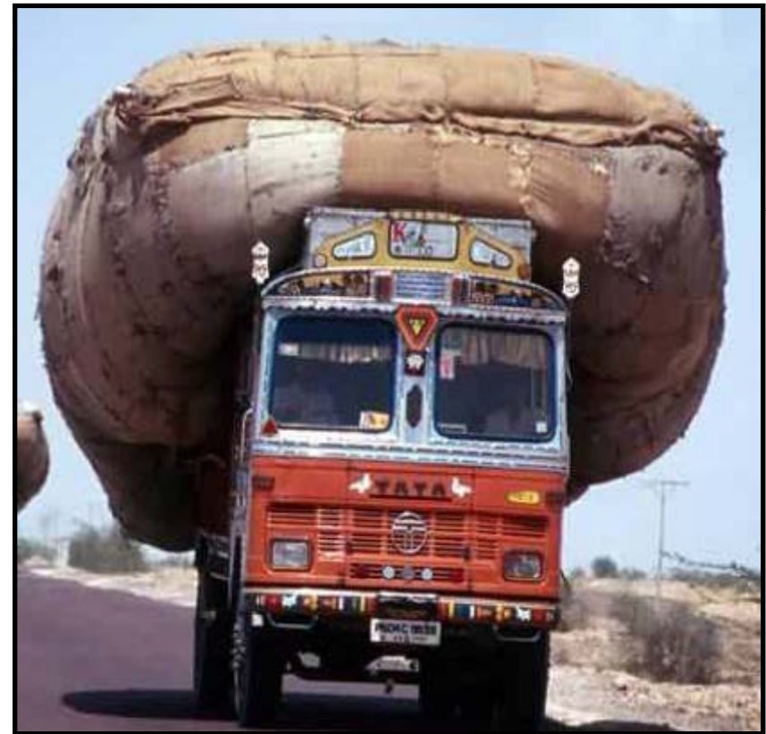
Overloading of Truck
