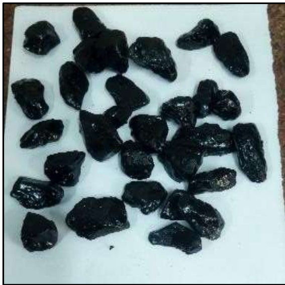
Aggregates coated with biobinder BEFORE BOILING TEST
