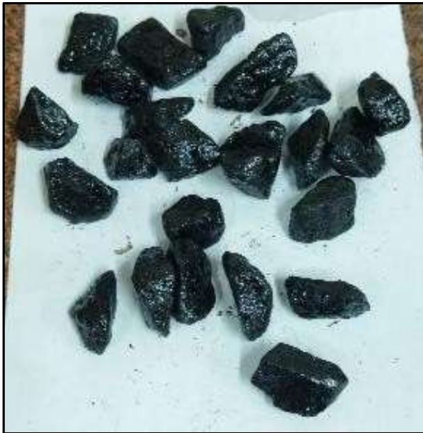
VG-40 COATED AGGREGATES AFTER BOILING: 99.7% Coating
