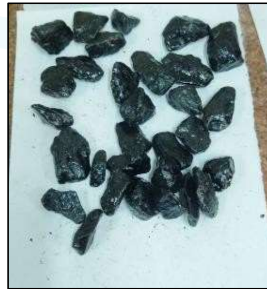
Aggregates coated with biobinder AFTER BOILING TEST
