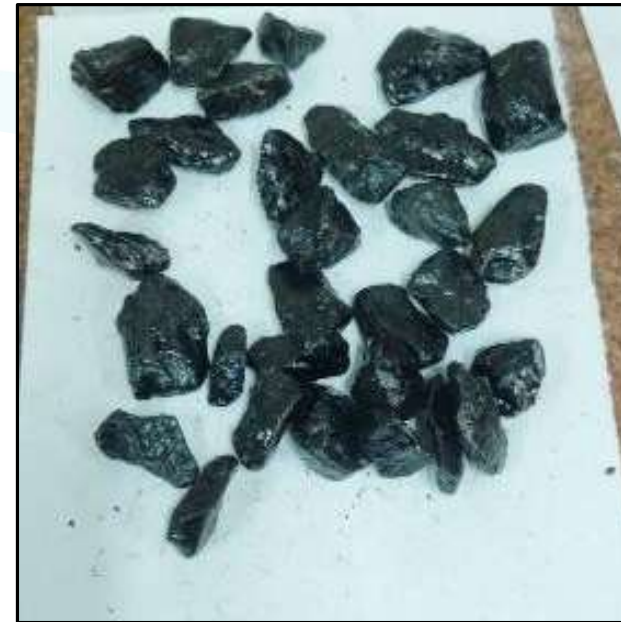
BIOBINDER COATED AGGREGATES AFTER BOILING: 99% Coating
