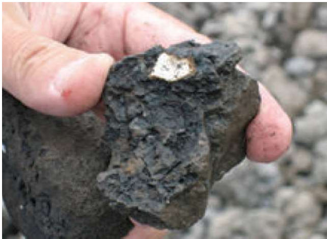
Free Lime Pocket in Slag
