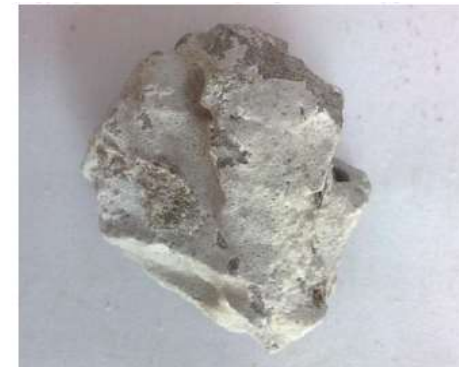
(c) Enlarged image of steel slag aggregate displaying the presence of coating of calcite
