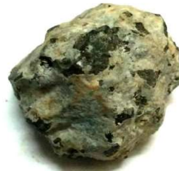
(c) Enlarged image of steel slag aggregate displaying the presence of coating of calcite
