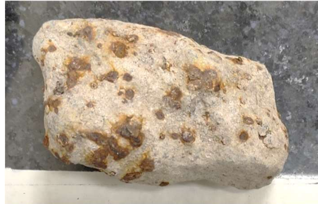
Corrosion in BOF Slag Aggregate
