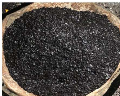
Asphalt Mix sample of waste plastic
