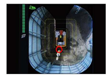
Recognizes intrusion in the machine's work area with alarm buzzer and a circle mark on the monitor to alert the operator.
