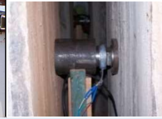
Special fixture arrangements for evaluation of longitudinal force
