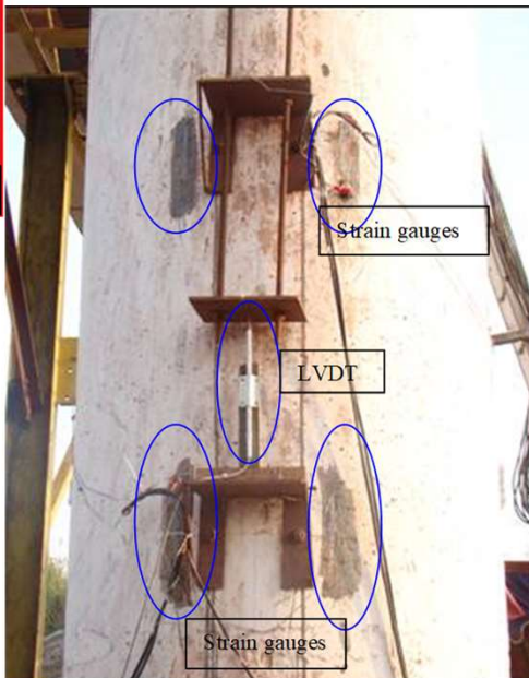
LVDT and strain gaging on piers
