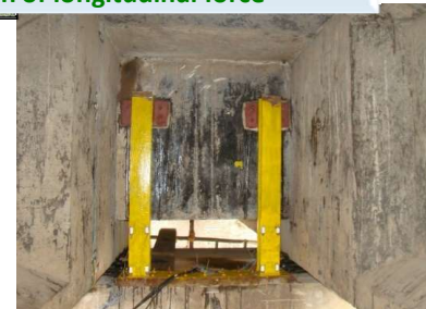
Special fixture arrangements for evaluation of longitudinal force
