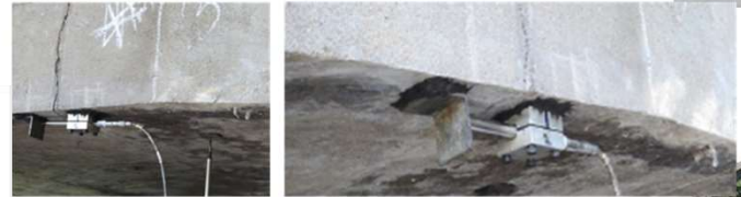
(d) Measuring the widening of existing cracks on the arch
