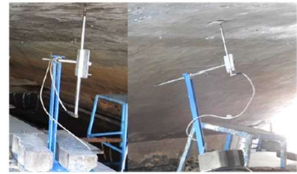
(b) Measuring the vertical deflection of the arch
