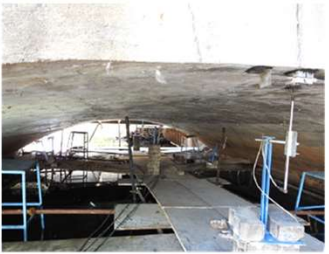
(a) Measuring the responses of the arch
