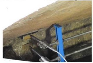
(c) Measuring the arch spread
