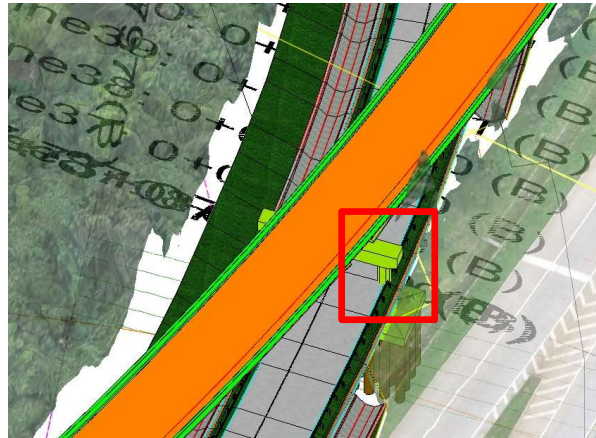
Pier misplaced on ramp
