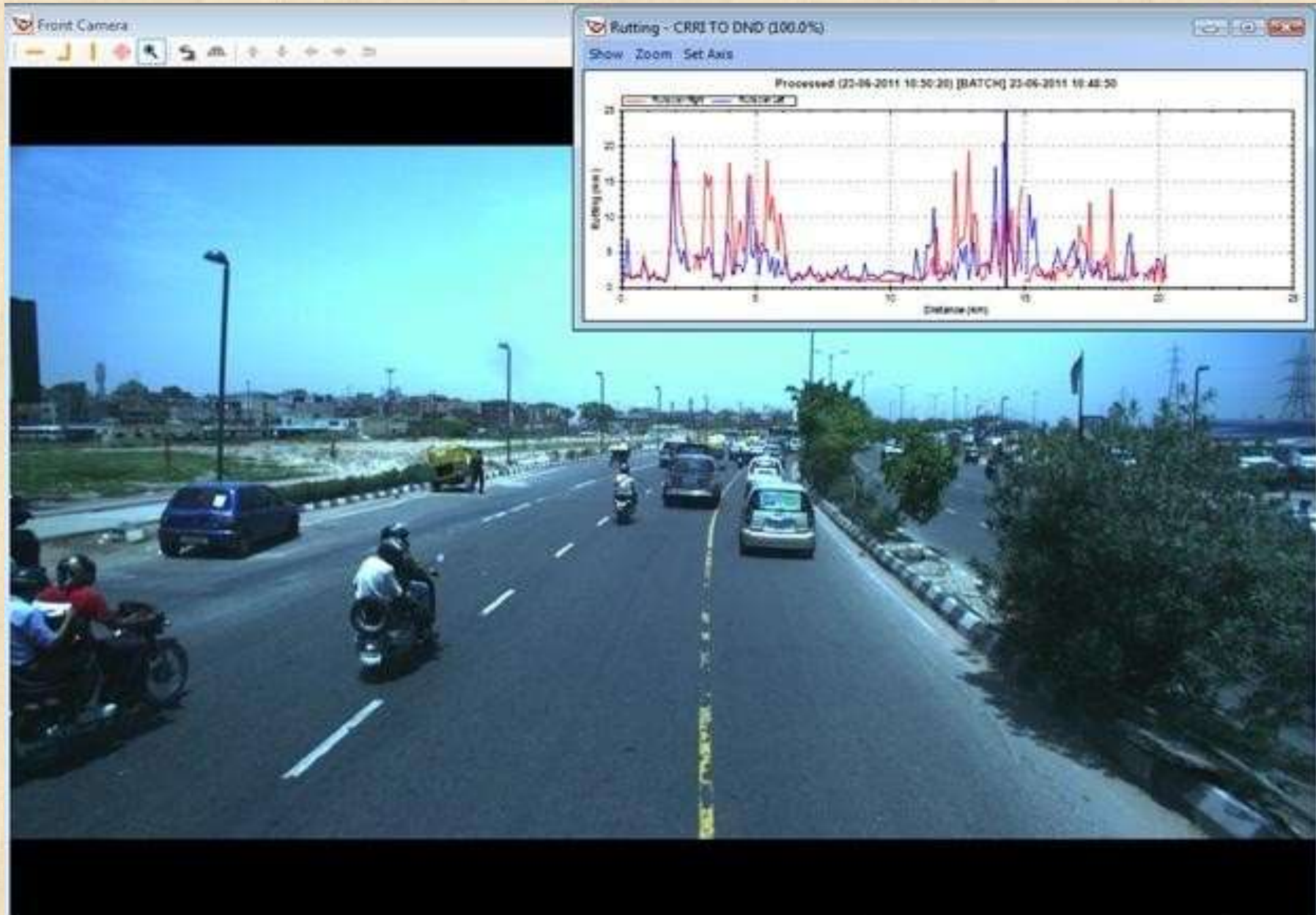
Comparison of Rut data with the Real Pavement Surface Condition (High Rut Depth)
