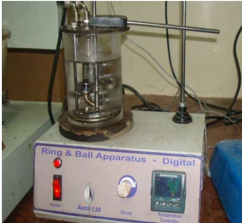
Ring Ball Apparatus with bath liquid Glycerin
