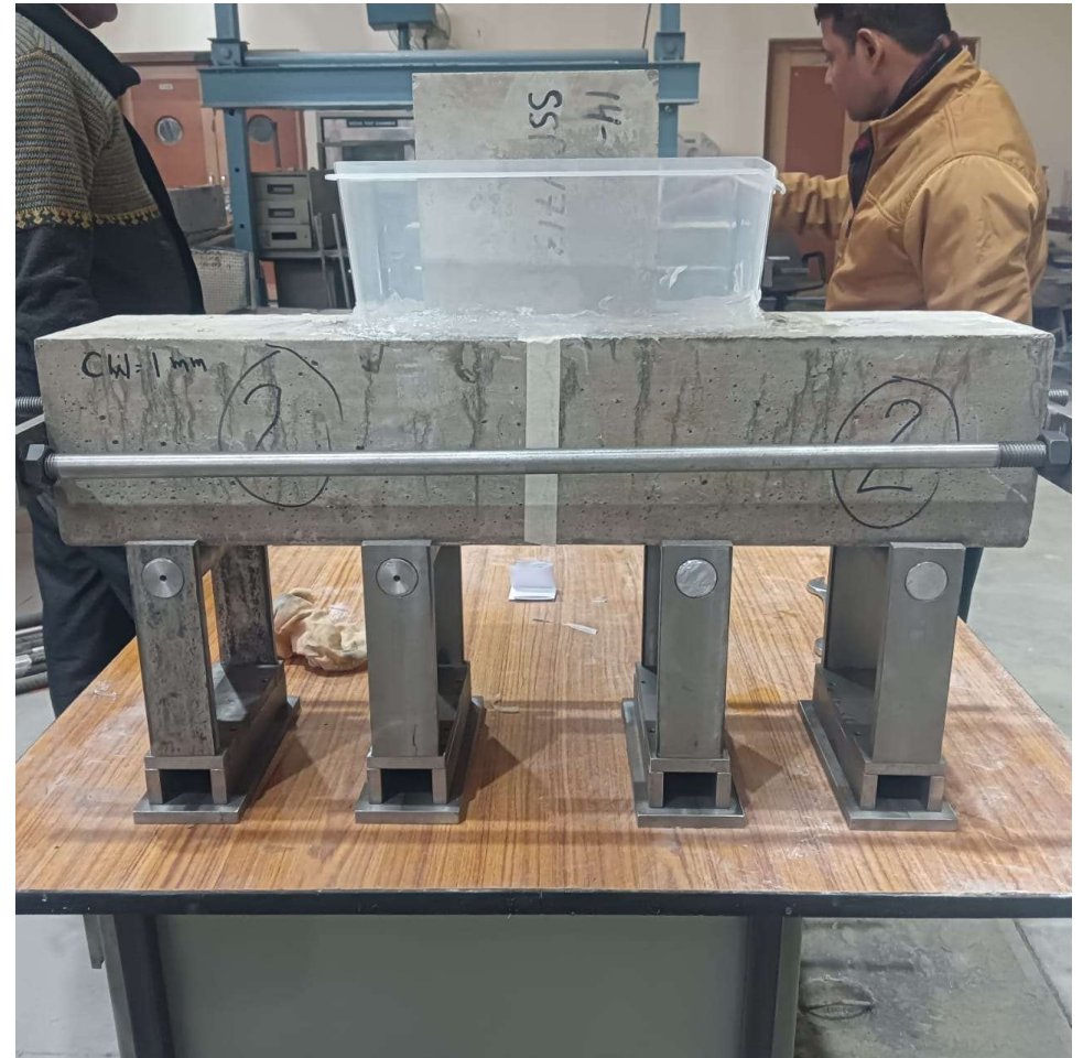
Potentiometric Titrator and Crack Sealing Test Setup.
