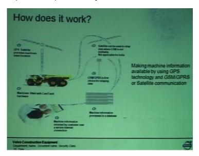
This is a brief illustration of how it works. The GPS Satellites provide the location of the machine, and the information that is on board in the electronics is collected and transmitted via GSM networks or GPRS networks. It is transmitted via these networks to the servers wherever placed. Right now, we have one in Sweden.
