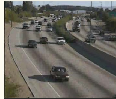
Speeds at or near FFS, Freedom to maneuver is noticeably restricted, Queues may form behind any significant blockage
