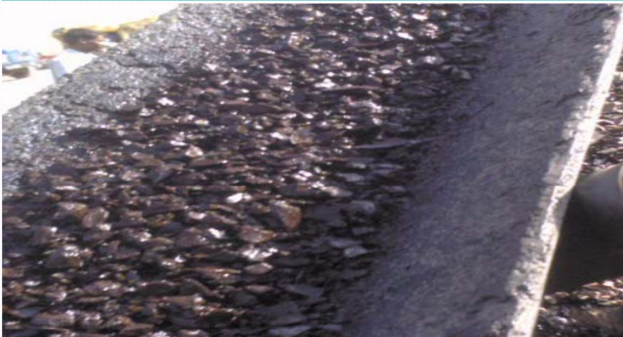
Cold Mix on Conveyer Belt
