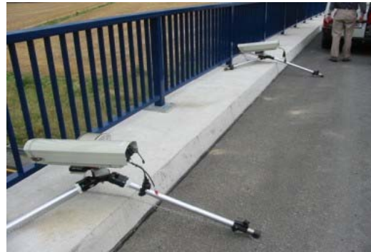
Video based speed measurement
