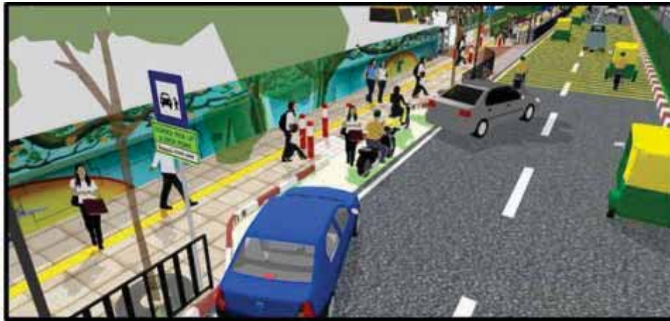
Pick and Drop Facility for Private Vehicles (The kerb stone is a deterrent)
