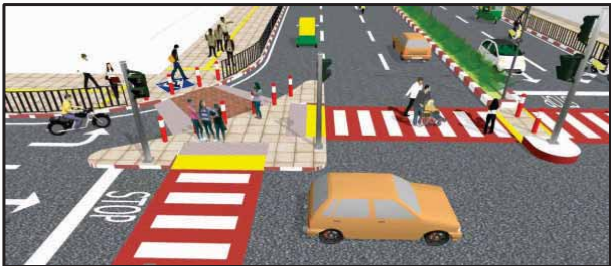
Refuge Island with safe space for pedestrians
