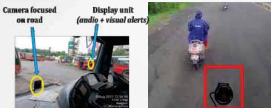
Figure 2: CAS unit installed in a bus; Typical Illustration of PCW warning generated due to 2-wheeler
